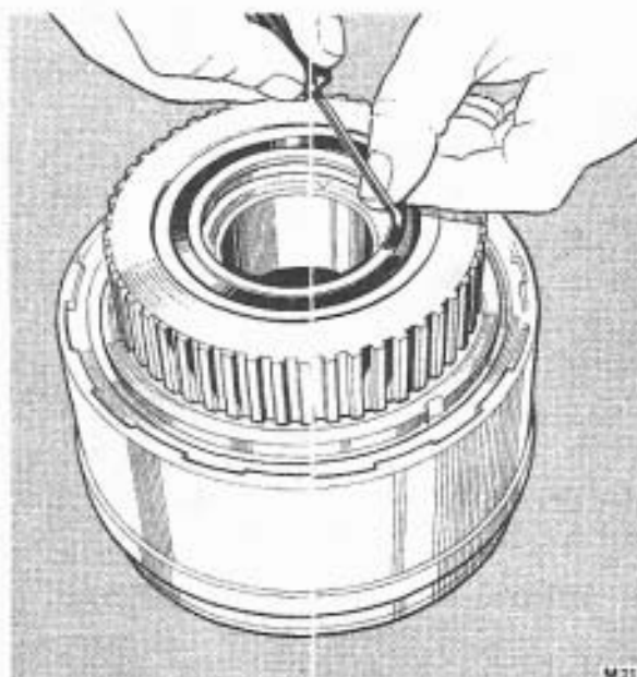
FIG. T104 REMOVING THE SPRAG RETAINING RING
