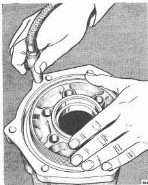
FIG. T88 REMOVING THE REVERSE CLUTCH PISTON
