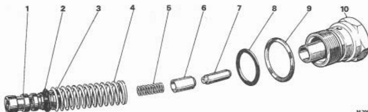
FIG. T67 PRESSURE CONTROL VALVE
