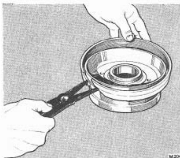
FIG. T86 REMOVING THE STATIONARY CONE
