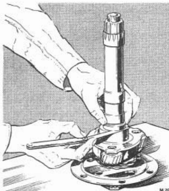
FIG. T89 CHECKING THE REVERSE PLANET CARRIER END FLOAT
