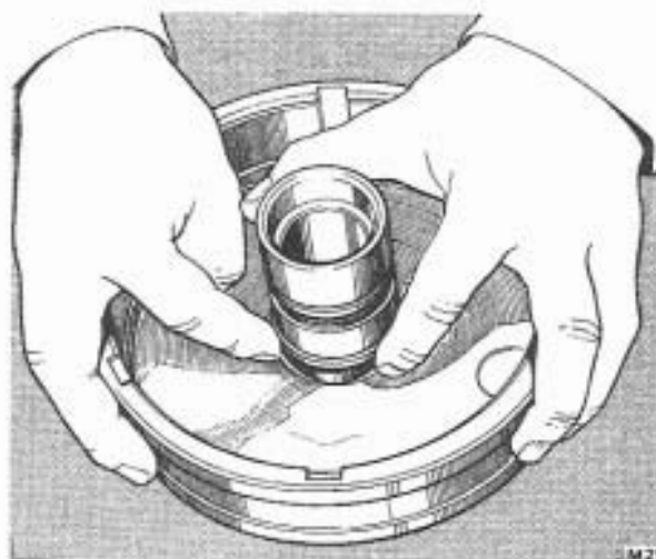
FIG. T108 FITTING THE OIL SEAL TO THE CENTRE CLUTCH DRUM ASSEMBLY
