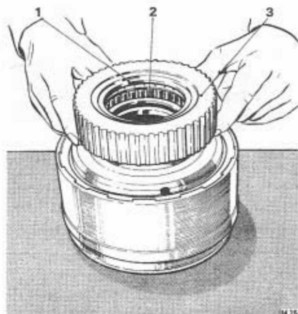
FIG. T113 FITTING THE SPRAG CLUTCH ASSEMBLY
